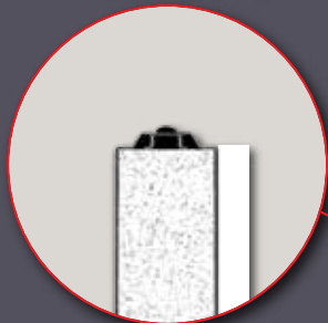
Tongue & Groove Weather Joint with Thermal Break
